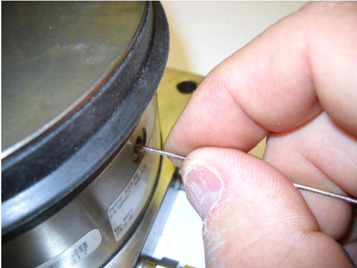
Figure No. 13 – Probing cell gauge port to determine piston position.
